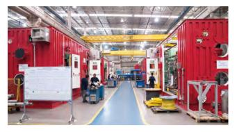
The Brazilian site in Jundiaí has become one of Sulzer's primary development, manufacturing, and distribution centers. Sulzer's test bed in Brazil is the largest pump test facility in the south hemisphere. With 13,800 V electrical supply installed, a sump depth of 11 m and a motor capacity up to 15,000 kW, this facility is able to test any centrifugal pump type from vertical to horizontal and submersible, single or multistage, within these technical limits. Among other products, the
