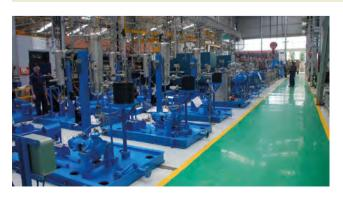
The facility in India handles stringent quality and testing requirements and supplies complex packaged pumps all over the world. Test bed capacity is 3.5 MW (50Hz/ 60 Hz) and 8 pumps performance testing at a time (depending upon size and motor ratings) is possible. Non-destructive testing such as liquid penetrant/magnetic particle/radiographic testing is also possible.
