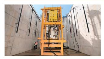
Sulzer has in Leeds one of the world's largest pump test beds for string testing gas turbine driven pump packages with an installed drive power of up to 30 MW.
