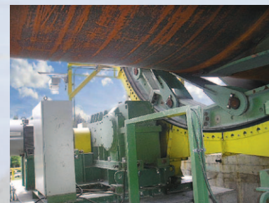
Girth Gears Output torque max 4000 kNm Gear ratio 4 - 16
